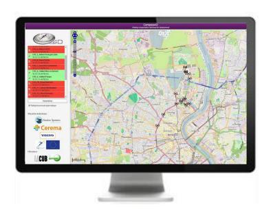
The FULLWEB platform permits the management and supervision of all the elements used for the operation of cooperative systems in Bordeaux. Especially the supervision of the Road Side Units and On Board Units but also the connections with the different data servers like TIPI for the road events and GERTRUDE for the information concerning the traffic lights. Another module permits the management of statistics and the evaluation of the efficiency of the system.
