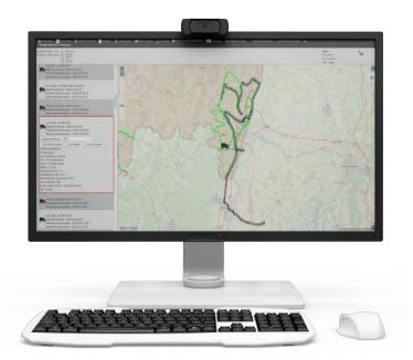
You can create, modify and complete road and events and plan road works and maintenance operations thanks to a selection tool. A non-real-time menu also allows to compile statistics and researches on completed events.
